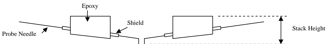
Figure 2, Cross section of coax epoxy spider.
